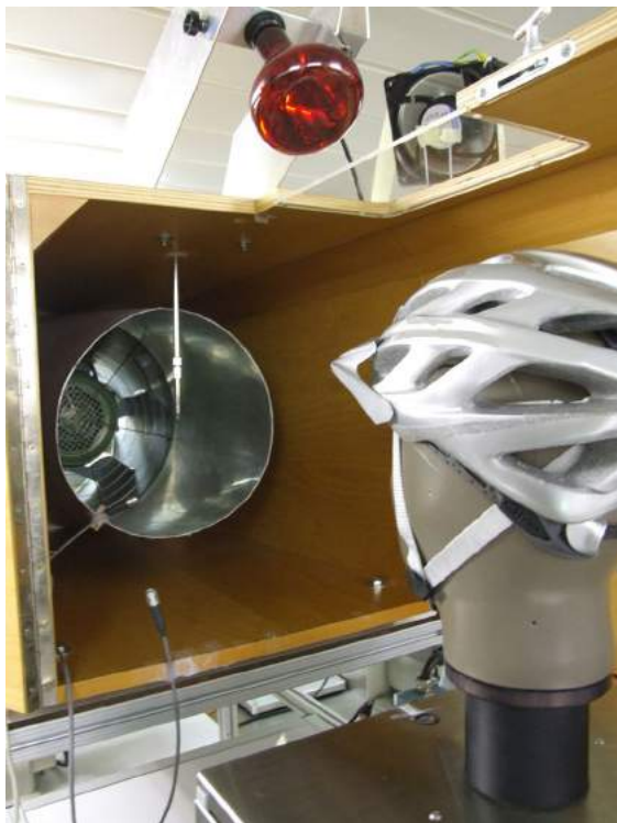
The advanced thermal manikin headform at Empa.
