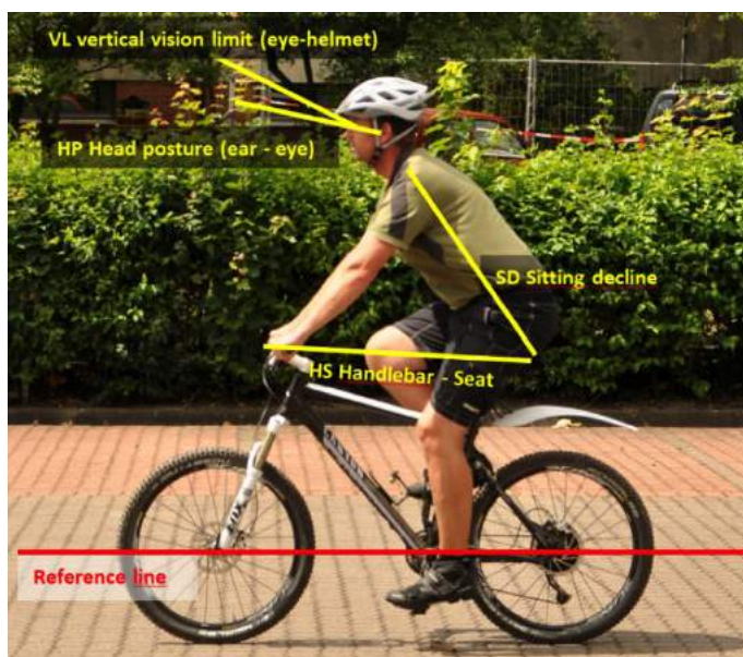
Establishment of angles relevant for seating geometry and vision limits
