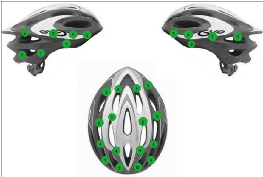
Figure 25: Damage matrix on helmets (smears / abrasions), representation of the location of damage to the helmet shell (specified as n-impact).
