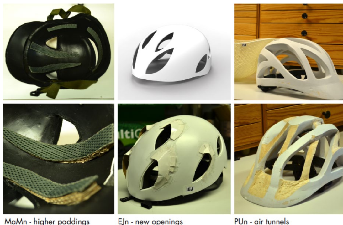
Figure 6. Some modifications of the design helmets ("n" means new solution of a helmet).
